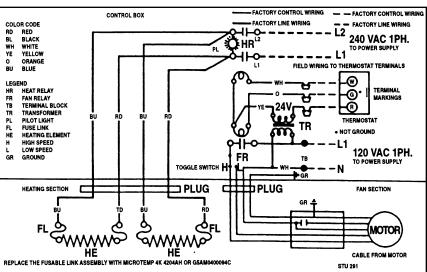
Figure 5 - Wiring Diagram
